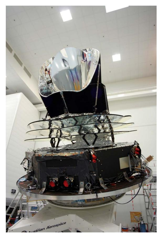
The only instrument flight item not integrated yet on the satellite is the HFI 4 K cooler, which is still under test at the Rutherford Appleton Laboratory. A spare unit has been mounted onto the satellite to allow environmental tests to proceed. The 4 K cooler has shown to be difficult to operate. A "Tiger Team" was appointed to address the problem. It
