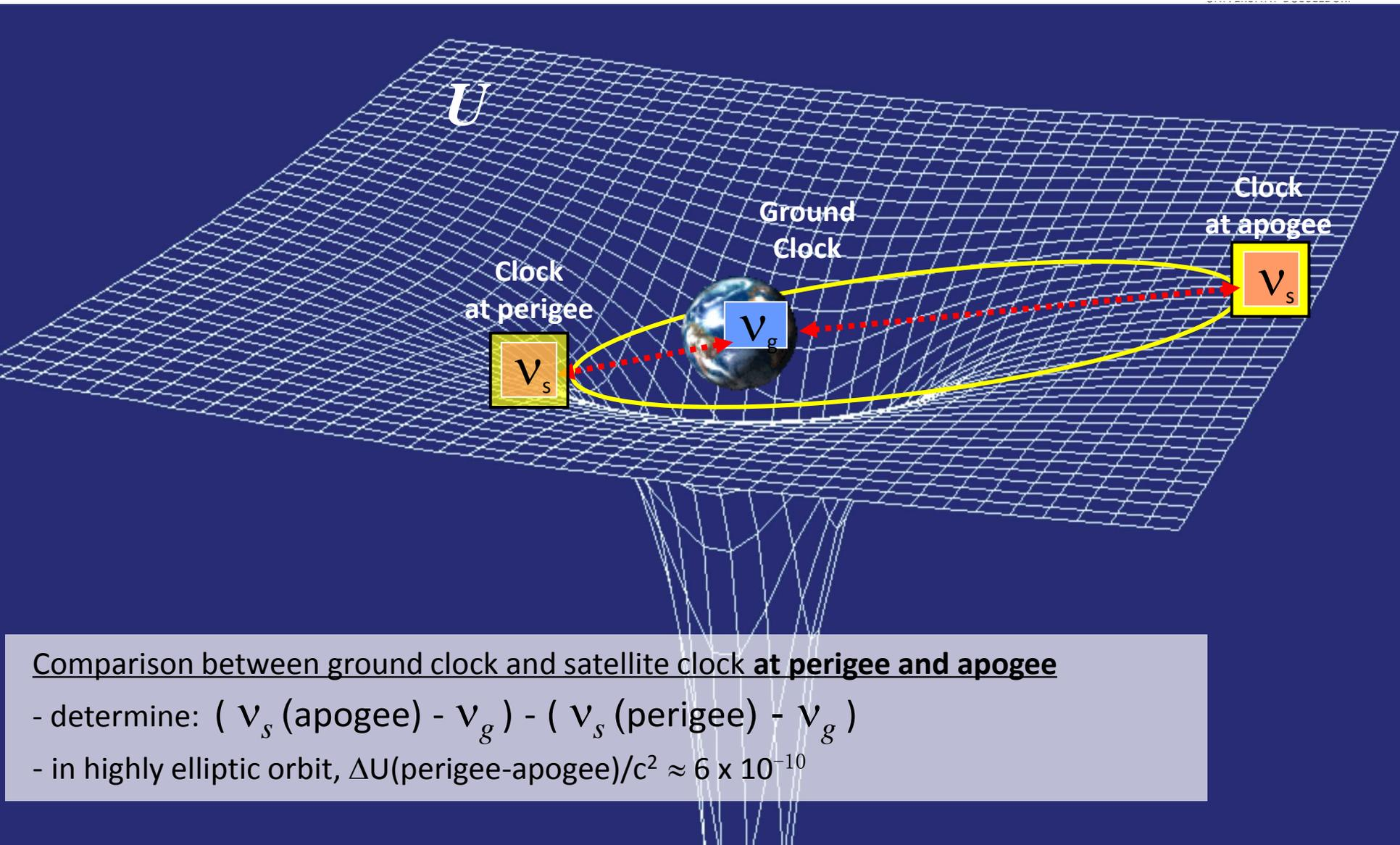
Comparison between ground clock and satellite clock at perigee and apogee
