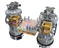
LISA Technology Package core assembly and inertial sensors http://sci.esa.int/lisa-pathfinder/56438
